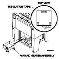
Check to be sure the discharge tubing is in its original position and discharge tube spacers are properly installed.  Disconnect the two terminals of the lighting harness. Connect the "Y" end of the pan and heater assembly harness (7849011) to the lighting harness as shown.
